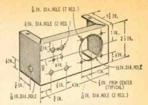
To insure easy construction, lay out chassis box holes as dimensioned above. Then remove burrs and apply several coats of spray paint for a professional appearance.
