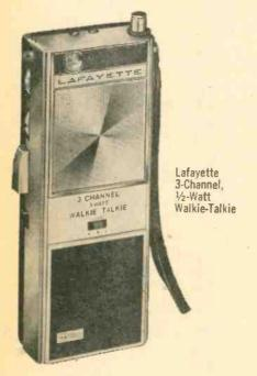
uV sensitivity, range boost modulation, provisions for tone call alert and 117-VAC operation with optional battery eliminator.
