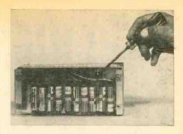
Rear apron of FETVM contains 10 batteries and coarse zero adjust control accessible through hole in rear cover.
