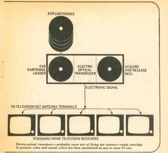
a special unperforated film, 8.75 millimeters wide. This master film is used to run off copies for purchase of EVR customers. Such copies are packaged in cartridges 7 in. in diameter and ½ in. thick—about the size of
