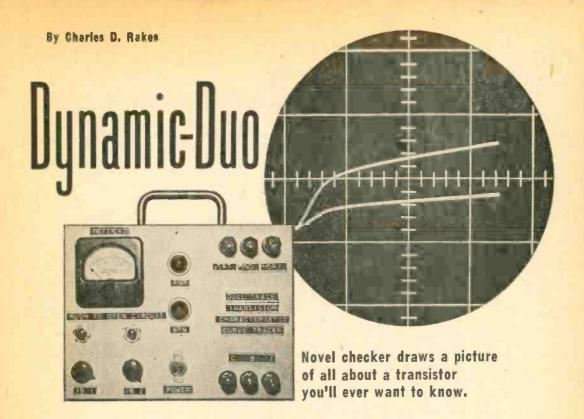
■ Dynamic Duo is a perfect name for our dual-trace transistor characteristic curve tracer. With this simple tester you can adjust and observe two I<sub>c</sub>/V<sub>ce</sub> curves of the same transistor on a scope simultaneously. And from this dual trace you can determine AC current gain (H<sub>fe</sub>), ideal base current for linear operation, and leakage current (I<sub>ceo</sub>). You can even match transistors for amplifier applications. Sound complicated? Not at all.
