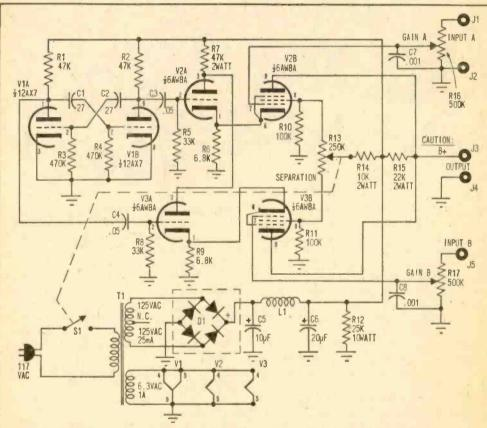
Schematic of Two-Timer shows straightforward approach to obtaining dual traces on a conventional single-trace scope. Unit is basically a high-speed electronic switch.
