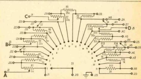
This is the schematic of the author's version of the load box; the string of power resistors, potentiometers, and series switches providing the ultimate in flexibility. At right, is the hookup employed in the knife-switch and monitoring meter circuits.
