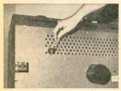
Remote speaker jack can be mounted in one of the ventilation holes in back of set, or 3/2-in, hole can be drilled to suit.
