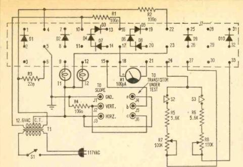
Fig. 3. Schematic diagram of Dynamic Duo transistor characteristic curve tracer.
