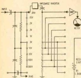
FETVM AC circuitry employs only two voltage divisions for input voltage to keep signal level to FET high.
