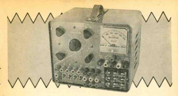
fraction of an ohm to more than 3700 ohms, with a power rating throughout in excess of 25 watts. Other features include built-in current-monitoring meter, fuses, and sufficient banana plug tie-points in the string of power resistors to provide a variety of series, series/parallel, and parallel connec-
